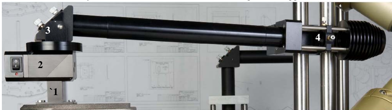
Figure 20 CO_2 laser beam delivery assembly.
